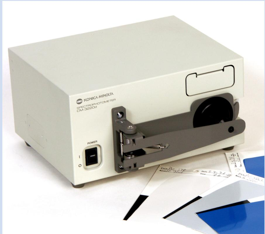
The **CM-3220d** is a very compact and rugged d/8 geometry instrument for POS applications with full data compatibility with all Konica Minolta CM-36xx and CM-2xxx models
